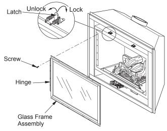
Figure 37 - Removing/Replacing Glass Door
